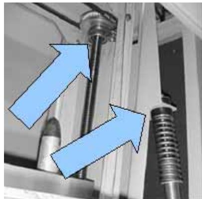
Remove all spilt paint from accessible parts (especially clamping plate spindles).
