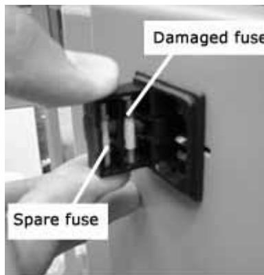
Remove mains connector and pull fuse tray outwards.
