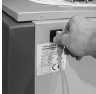
Connect the SK300 to the power mains before closing the door.
