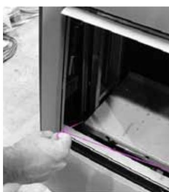
Pull out cord to remove frame lock's loose parts.
