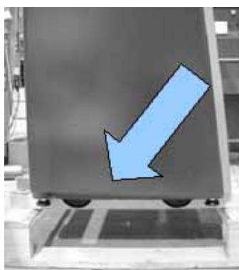
Remove box and plastic foil. Note the frame lock bolts on either side of the machine.
