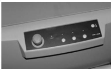
Turn the emergency stop clockwise to unlock: the power led is lighted-ON.
