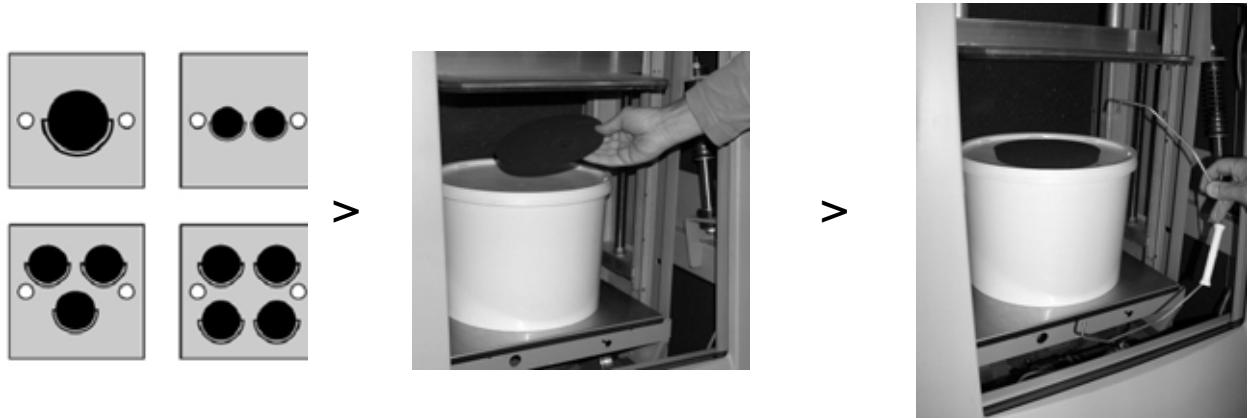
Place one or more containers at gravitational center of the can table, between the spindles.
